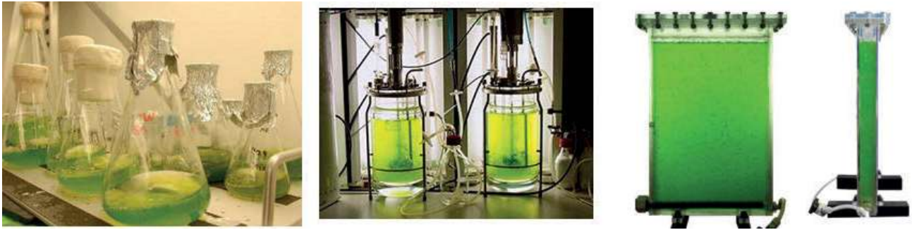
Figure 7 Three examples of contained production of algae: Erlenmeyers, fermenters and flat panel reactors
